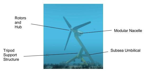
Figure 2: A schematic of the 300kW device
